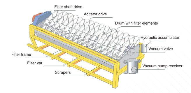
Best design of agitator, shaft, agitator drive and filter vat provides uniform mixing of high density slurries and therefore maximizes process performance.
