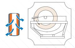
The design of the CDF filter provides ultrasonic cleaning of ceramic filter elements, which ensures the most efficient performance of the ceramic filter elements.
